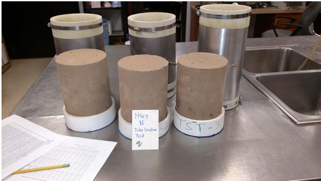
Figure 2.5.3.2 – Tube Suction Test Setup (Photo Credit – Chase Henrichs)
