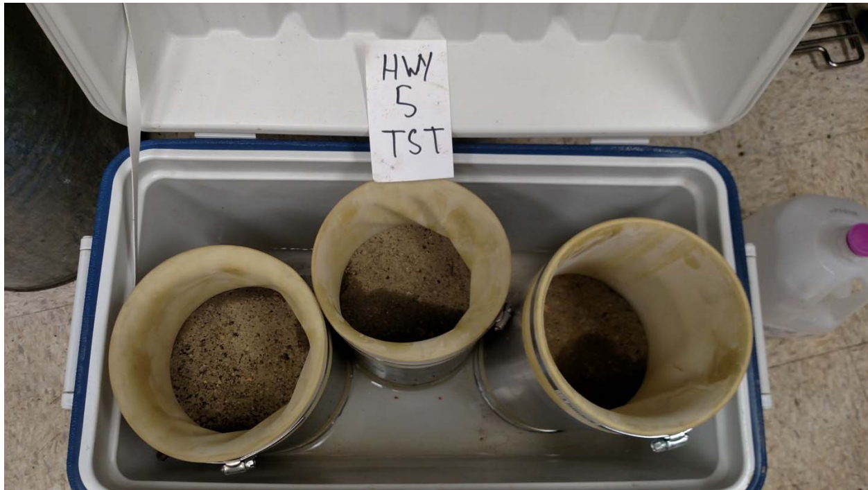
Figure 2.5.3.3 – Tube Suction Test (Photo Credit – Chase Henrichs)
