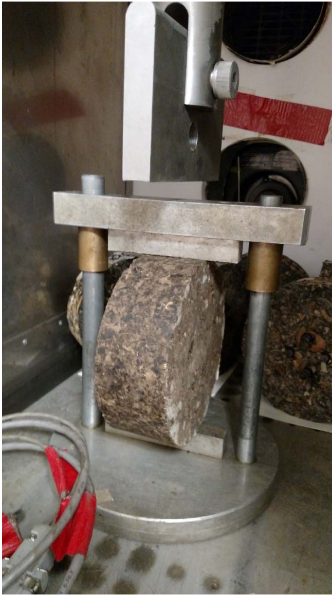
Figure 2.5.3.1 – Indirect Tensile Strength Test (Photo Credit – Chase Henrichs)
