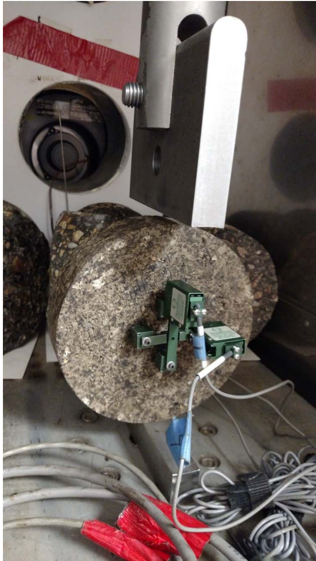
Figure 2.5.1.1 – Dynamic Modulus and Creep Compliance Testing Configuration (Photo Credit – Chase Henrichs)
